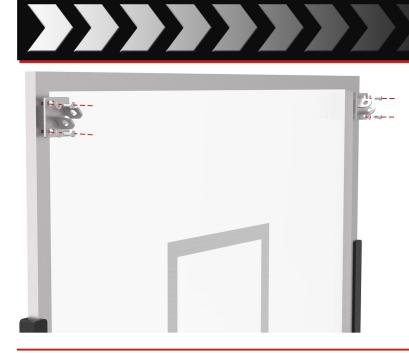
4,Install backboard connection plate: using M10\*20mm bolts, washer to fix the plate on the backboard.
