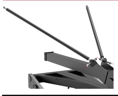
3,Install top rod: using M20\*60mm bolts, washer, spring washer, nuts to fix the plate on the arm.
